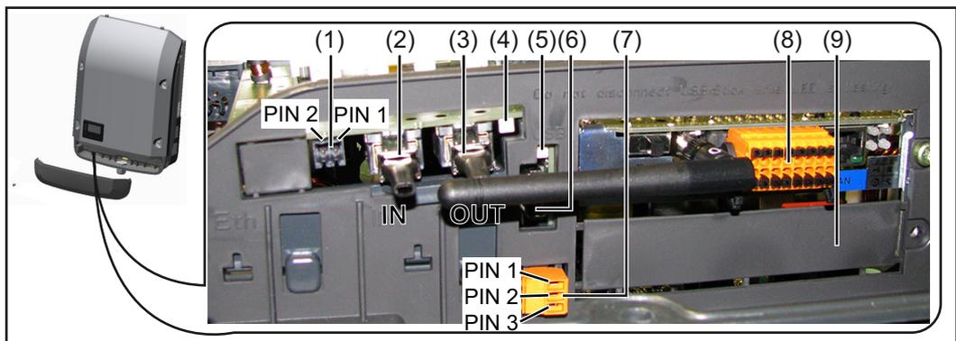
Depending on the model, the inverter may be equipped with the Fronius Datamanager plug-in card.
