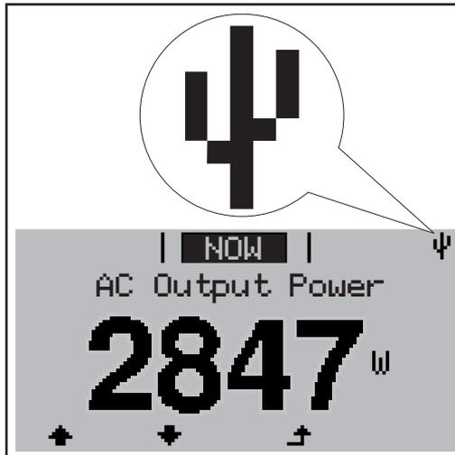
If the inverter detects a USB flash drive, the USB symbol will appear in the top right corner of the display.
